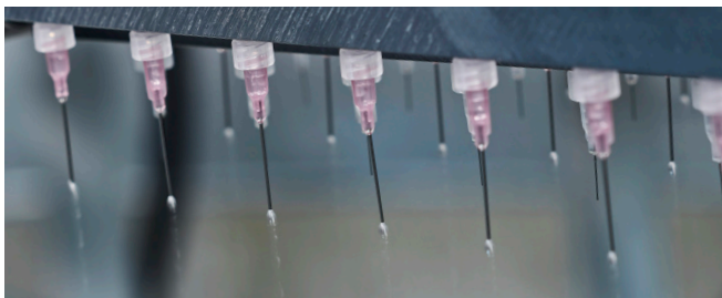
600 nozzles simulate realistic rainfall with adjustable droplet size.
